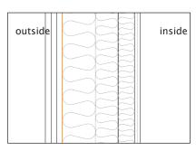
DAFA RooFoil 200 used as a wind barrier with a ventilated cavity behind the rainshield
