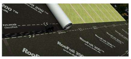
DAFA RooFoil 200 is installed with a minimum overlap of 150 mm and free joints are taped using DAFA UV tape.
