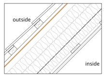
DAFA RooFoil 200 used as roof decking with ventilation between insulation and roof decking.
