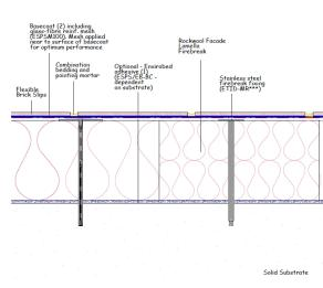
Figure 2 - Horizontal firebreak detail - plan view
