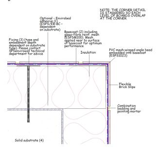
Figure 3 - Window reveal detail
