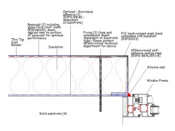
Figure 5 - Horizontal movement joint detail
