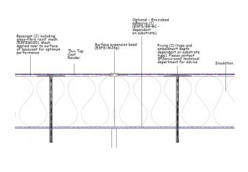
Figure 2 - Horizontal firebreak detail - plan view
