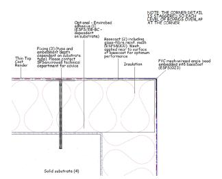
Figure 3 - Window reveal detail
