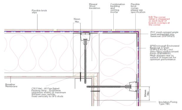
Figure 2 - Horizontal firebreak detail - plan view
