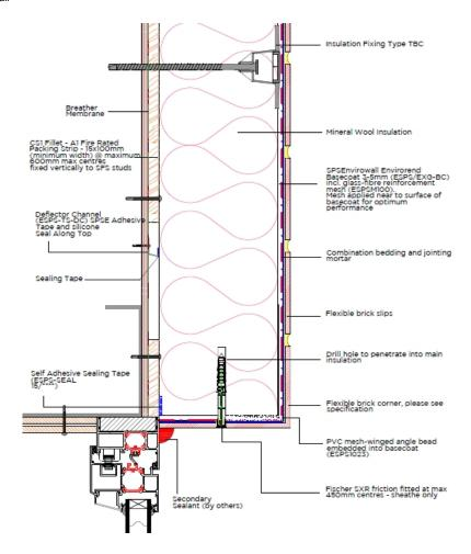
Figure 6 - Horizontal movement joint detail
