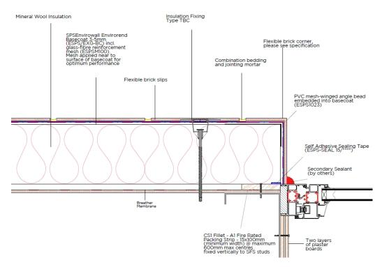
Figure 4 - Vertical firebreak detail
