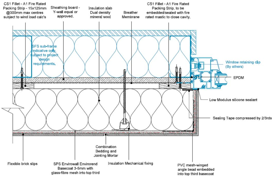
Diagram 5 - Horizontal fire barrier detail
