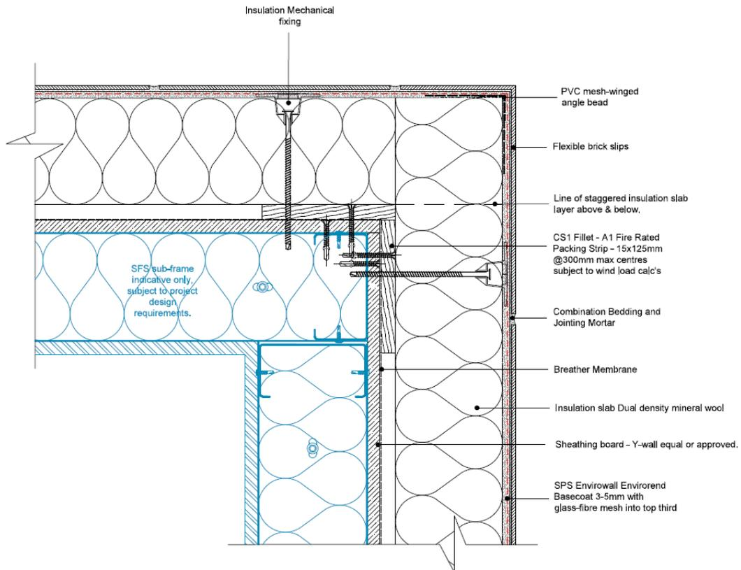
Diagram 3 - Vertical fire barrier detail
