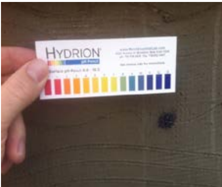
Step 5. Measure colour against chart, if it is above 8 wait some time and test again
