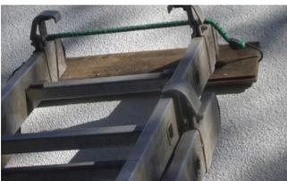
When using ladders for access, it is important to ensure that the ends of the ladder in contact with the render has a load spreader attachment to ensure there are no pint loads that may damage the render coating.
