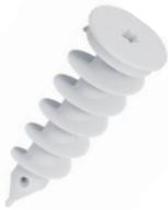
For new fittings less than 5kg in weight, this can be done using SPS Spiral Anchors that are fixed through the render and sealed using a compressible washer and / or mastic sealant.
